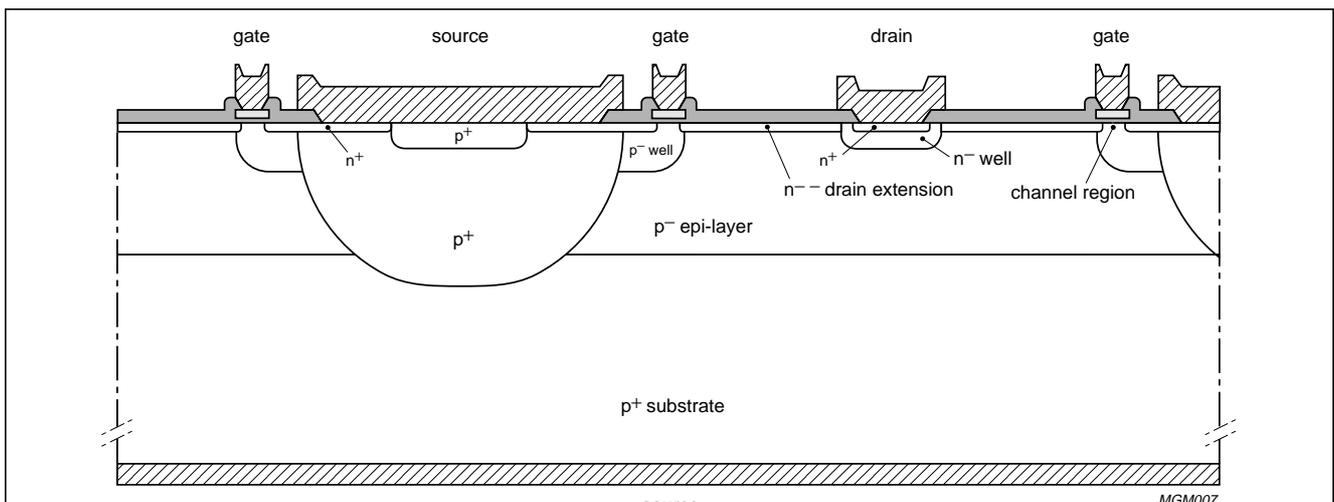
Fig.1-11 Cross-section of an LDMOS transmitting transistor. The *length* of the gate (the channel length) is in the plane of the paper; the channel *width* is into the plane of the paper.
