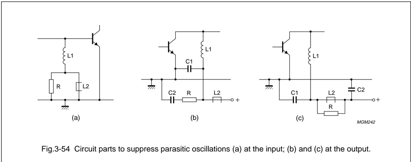
Fig.3-54 Circuit parts to suppress parasitic oscillations (a) at the input; (b) and (c) at the output.
