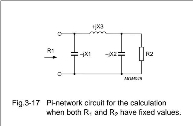
Fig.3-17 Pi-network circuit for the calculation when both  $R_1$  and  $R_2$  have fixed values.
