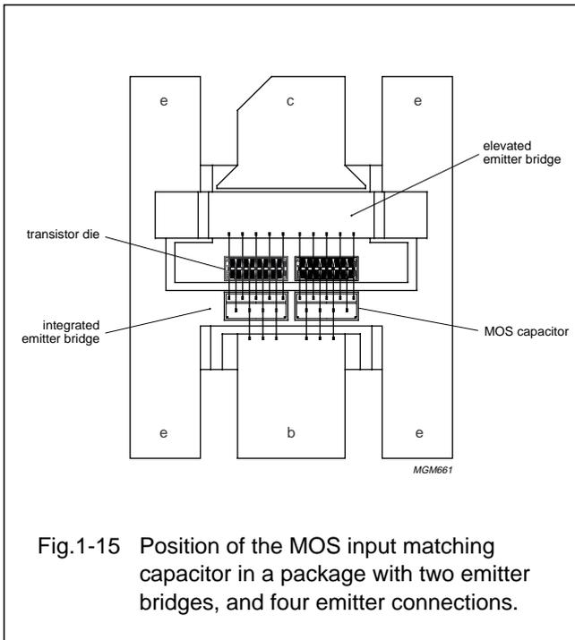
Fig.1-15 Position of the MOS input matching capacitor in a package with two emitter bridges, and four emitter connections.
