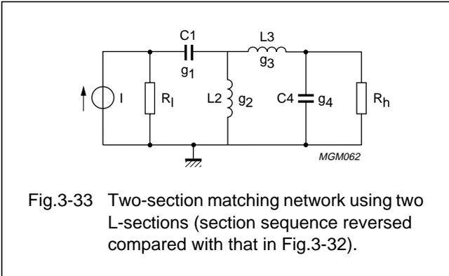
Fig.3-33 Two-section matching network using two L-sections (section sequence reversed compared with that in Fig.3-32).
