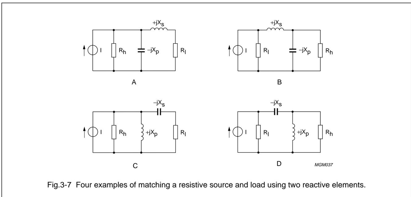
Fig.3-7 Four examples of matching a resistive source and load using two reactive elements.
