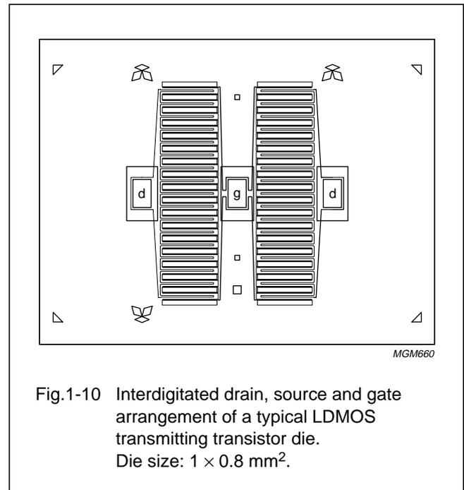
Fig.1-10 Interdigitated drain, source and gate arrangement of a typical LDMOS transmitting transistor die. Die size: 1 x 0.8 mm².
