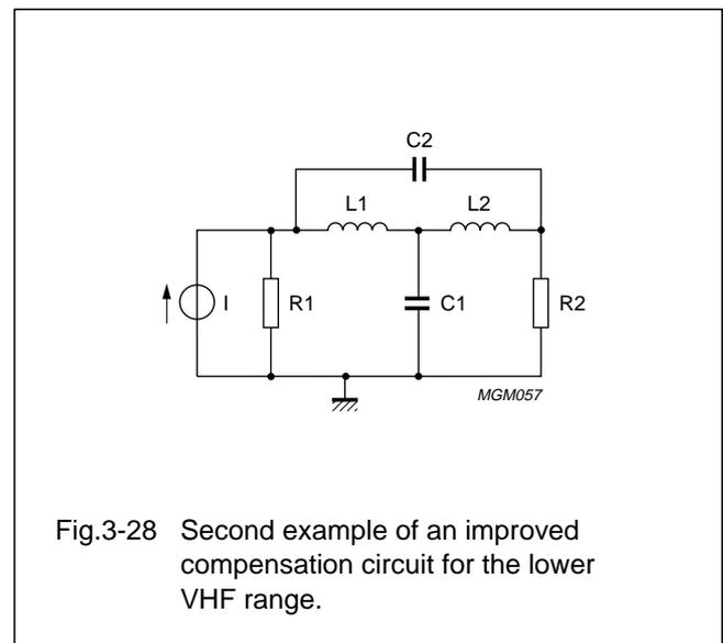
Fig.3-28 Second example of an improved compensation circuit for the lower VHF range.
