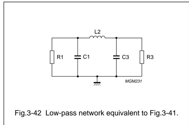
Fig.3-42 Low-pass network equivalent to Fig.3-41.
