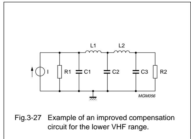
Fig.3-27 Example of an improved compensation circuit for the lower VHF range.
