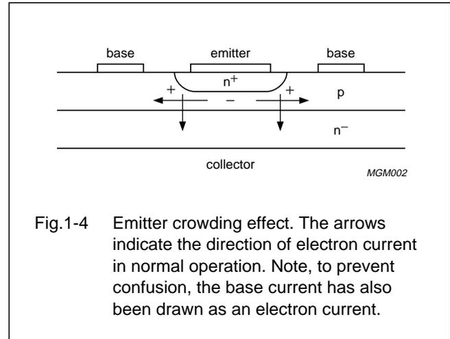
Fig.1-4 Emitter crowding effect. The arrows indicate the direction of electron current in normal operation. Note, to prevent confusion, the base current has also been drawn as an electron current.
