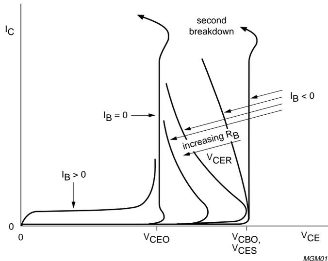
Fig.2-2 Definition of breakdown voltages.
