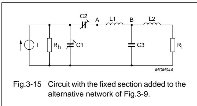
Fig.3-15 Circuit with the fixed section added to the alternative network of Fig.3-9.
