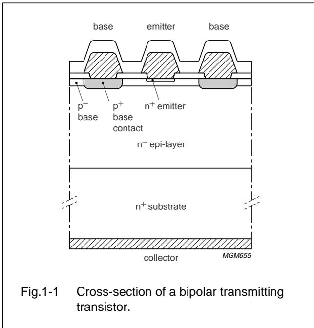
Fig.1-1 Cross-section of a bipolar transmitting transistor.
