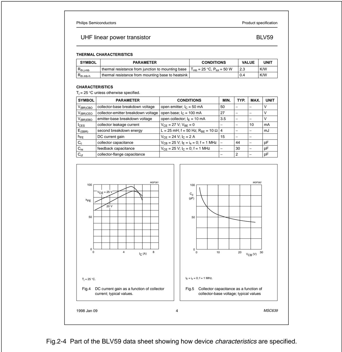
Fig.2-4 Part of the BLV59 data sheet showing how device characteristics are specified.
