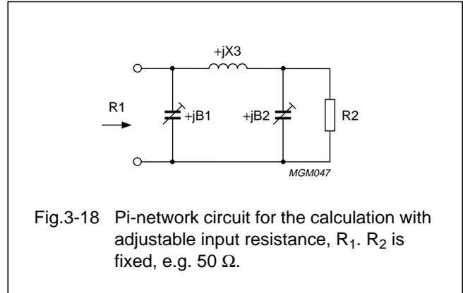
Fig.3-18 Pi-network circuit for the calculation with adjustable input resistance,  $R_1$ .  $R_2$  is fixed, e.g. 50  $\Omega$ .
