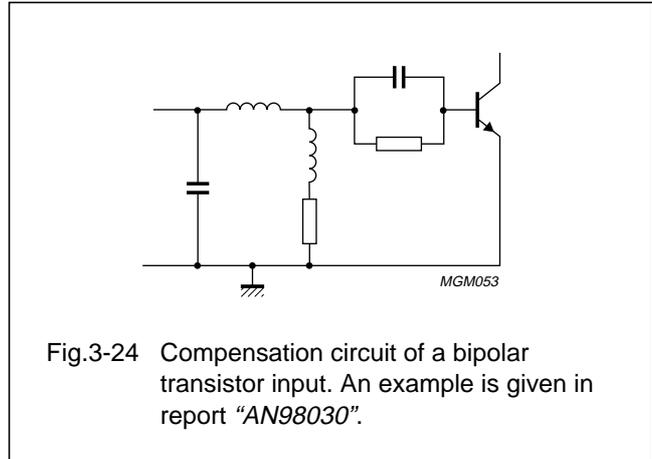
Fig.3-24 Compensation circuit of a bipolar transistor input. An example is given in report "AN98030".
