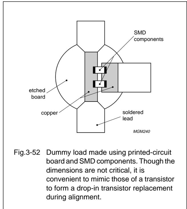
Fig.3-52 Dummy load made using printed-circuit board and SMD components. Though the dimensions are not critical, it is convenient to mimic those of a transistor to form a drop-in transistor replacement during alignment.
