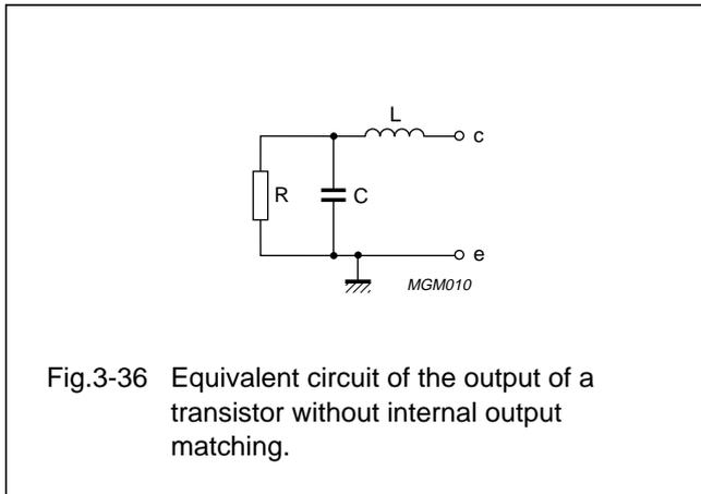
Fig.3-36 Equivalent circuit of the output of a transistor without internal output matching.
