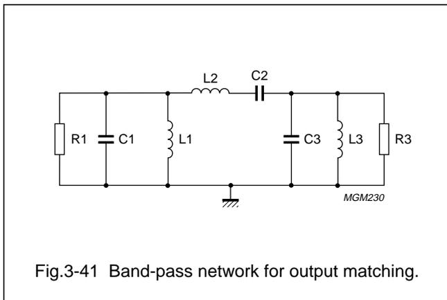
Fig.3-41 Band-pass network for output matching.
