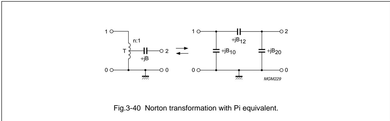
Fig.3-40 Norton transformation with Pi equivalent.
