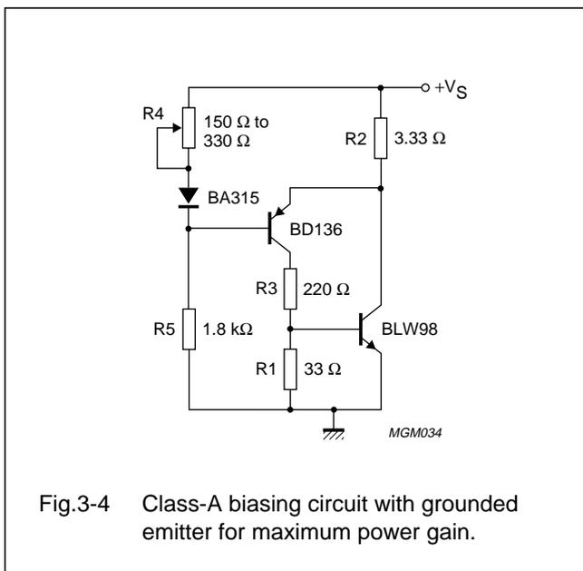
Fig.3-4 Class-A biasing circuit with grounded emitter for maximum power gain.
